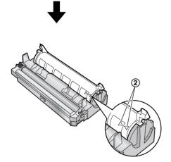
6 Remove the used cartridge (1) from the drum unit (2).
